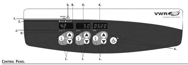
The front panel of the Incubating Orbital Shaker contains all the controls and displays needed to operate the unit.
